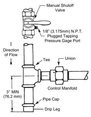
Supply Line Connection to Burner
