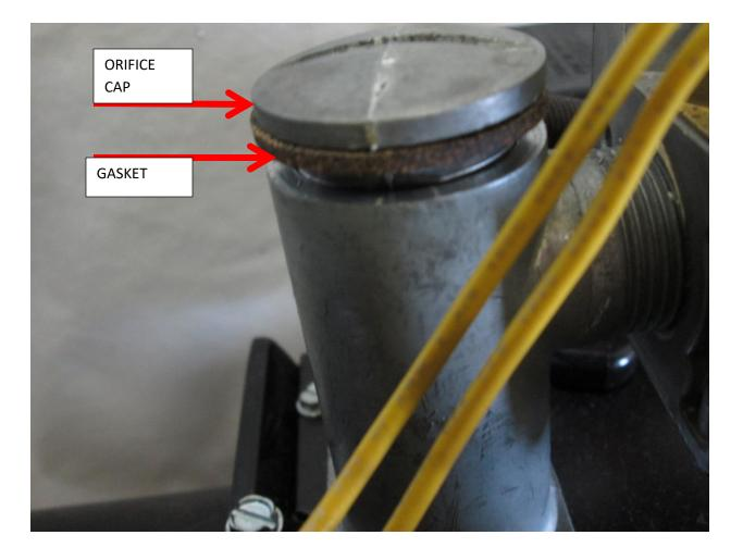
Figure 13: HSG Cap with Gasket on Manifold
