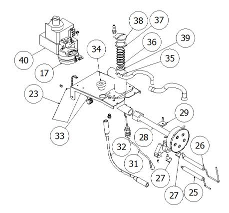
Figure 31: Gun Assembly Exploded
