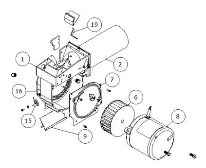
Figure 30: Motor Assembly Exploded
