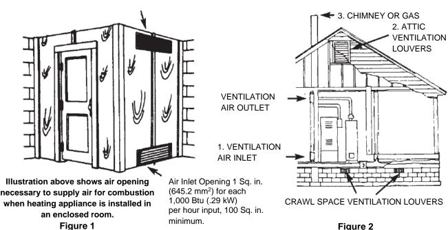
**NOTE ON FIGURE 2**: Ducts used for make-up air may be connected to the cold air return of the heating system only if they connect directly to outdoor air. Attic Ventilation Louvers are required at each end of attic with alternate air inlet No. 1.
