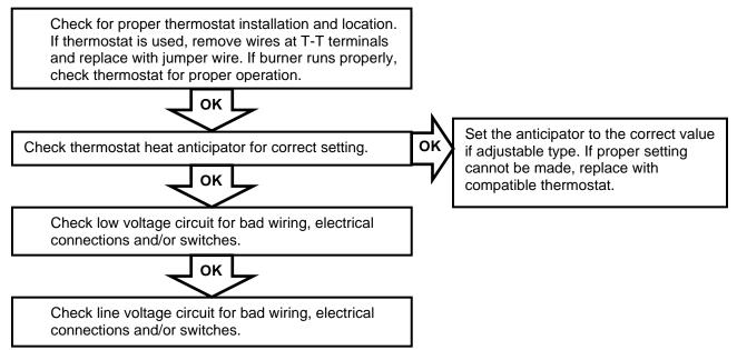
NOTE: When the thermostat wires terminate on the HSG primary control box "T" terminals, the heat anticipator setting value for the HSG burner is determined by adding the primary control current to the gas valve current. The result is the anticipator setting. (Example: 0.2 + 0.6 = 0.8 amps).
