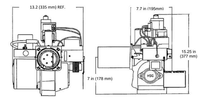
Figure 33: Outer Dimensions of HSG Series Burner
