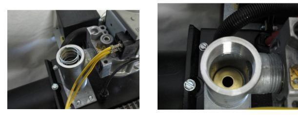
Figure 14: HSG Cap with Gasket Removed and Spring Removed
