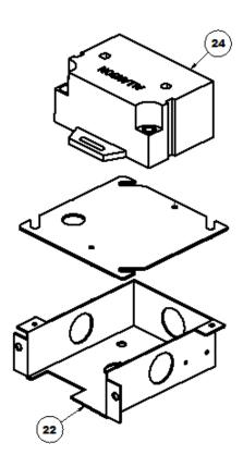
Figure 29 continued: Junction Box Assemblies Exploded
