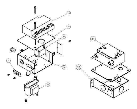
Figure 29: Junction Box Assemblies Exploded
