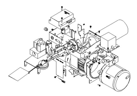
Figure 32: HSG Series Burner Exploded
