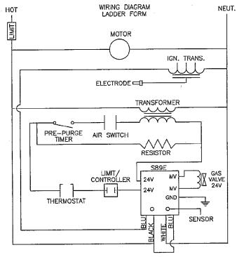
Figure 27: Wiring Diagram for Burners with Honeywell S89E Control
