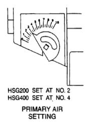
Figure 18: Air Settings for Initial Start Up
