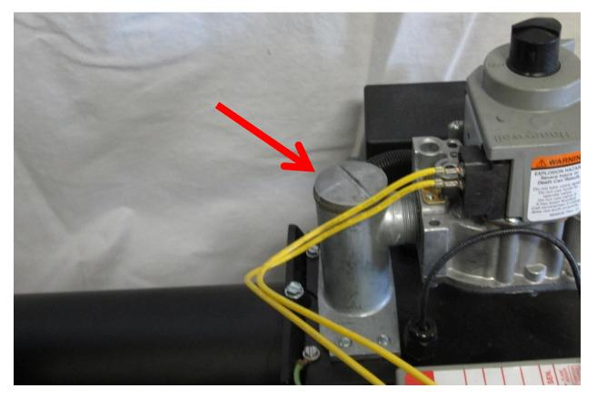
Figure 12: HSG Manifold
