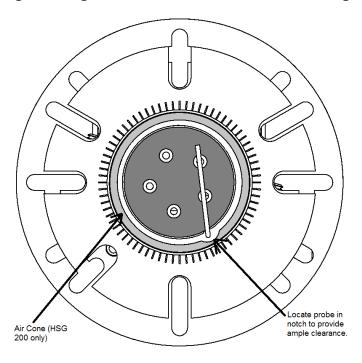
Figure 22: Burner Face and Flame Sensor Probe Location
