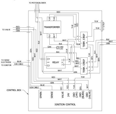
Connect to 120 Vac line voltage here. These wires to be supplied by installer.
