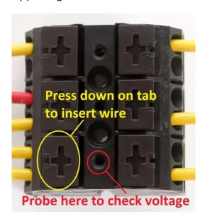
A closeup of a 63592-003 terminal block. Ports are connected in pairs on each side. Each pair is also connected to the pair on the opposite side.
